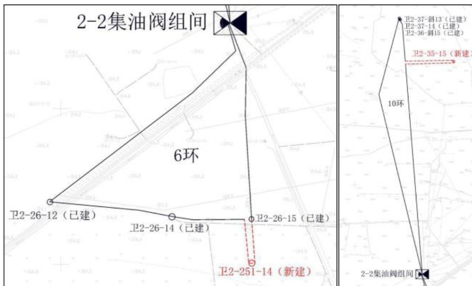
图3.5-3 2-2#阀组间集油管网布局
